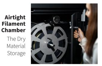
The sealed filament chamber stores two filament spools in an environment shielded from external influences. Drying cartridges further minimize humidity, allowing sensitive materials to be stored at a consistent dryness level.
